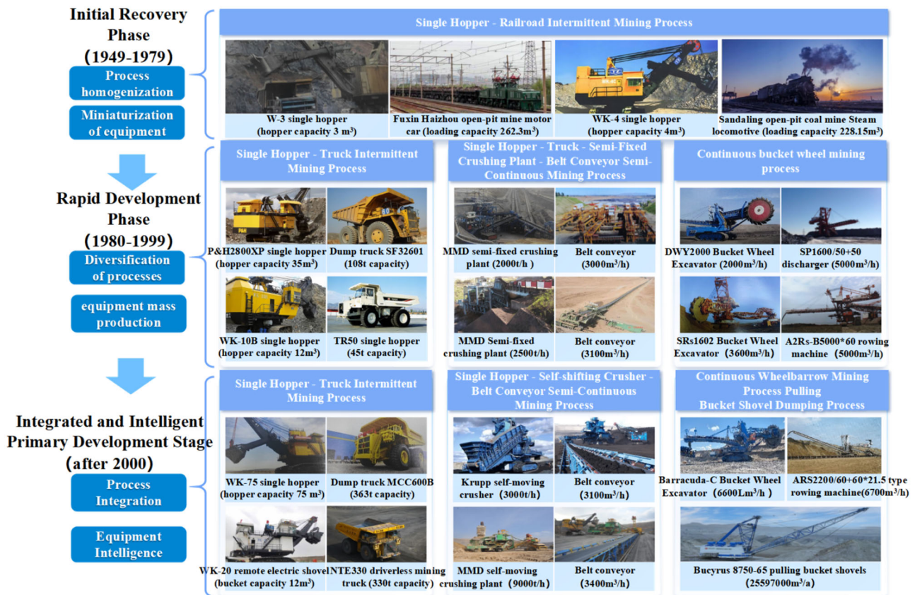
FIG 5 – Representative mining techniques and equipment at different development stages of open pit coalmines.
